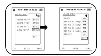
Press any button to cancel the alarm in physiological alarm state and this method brings no affection to the next alarm. To close alarm in 【ALARM SETUP】 will disable the alarm function until switch alarm on.
